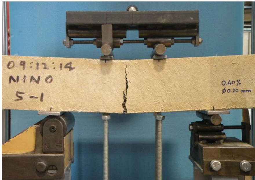
Figure 7: Flexural failure of FRC prism (mix C2 with 0.40% of \text{Ø}0.25 \text{ mm} HDPE fibres).
