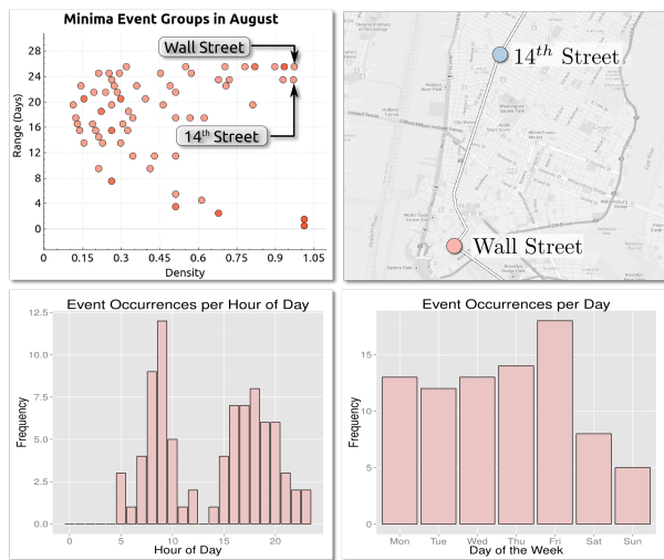
Fig. 11. Frequent minima events for August 2013 for the south bound 3 trains. Two of the event groups in Region II of the event group distribution view (daily events) corresponds to the Wall Street and the 14 th Street stations. Frequency distribution of events in the minimum event group corresponding to Wall street station indicates that this event predominantly occurs during rush hours, i.e., between 8 and 10am and between 4 and 8pm. Also note that the frequency of this event is higher on weekdays than on weekends.
