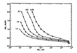
Figure 7 Life reduction caused by dents as a function of the relative slope  $(f_Z/f_X)$  for different values of  $f_X$ ,  $p_h = 2.5$  GPa, b = 0.25 mm, smooth contact life is  $0.4802 \frac{10^6}{10^6}$ .
