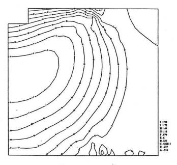
Figure 2c Residual hydrostatic stress below indentation; shown is the central square of 0.25 mm.
