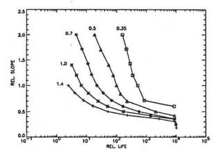
Figure 6 Life reduction caused by dents as a function of the relative slope  $(f_Z/f_X)$  for different values of  $f_X$ ,  $p_h = 3.0$  GPa, b = 0.30 mm, smooth contact life is 0.8513  $10^4$ .
