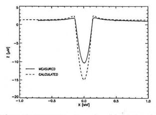
Figure 2a Comparison of experimental and theoretical dent profile.
