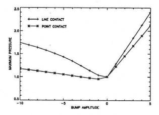
Figure 4 Comparison of maximum pressure between dented line and point contact, as a function of the amplitude. A < 0: dent, A > 0: bump,  $p_h = 3.0$  GPa, b = 0.3 mm,  $\lambda = 0.5$  mm.
