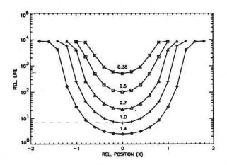
Figure 5 Life reduction as a function of the dent position relative to the centre of the contact, for a set of dents ( $f_X = f_Z = 0.35$ , 0.50, 0.70, 1.0, 1.4). Contact conditions:  $p_h = 3.0$  GPa, b = 0.3 mm, smooth contact life = 0.8513 10<sup>4</sup>.
