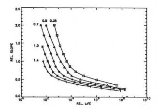
Figure 8 Life reduction caused by dents as a function of the relative slope  $(f_Z/f_X)$  for different values of  $f_X$ ,  $p_h = 2.0$  GPa, b = 0.20 mm, smooth contact life is 0.2459  $10^9$ .
