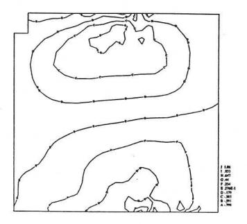
Figure 2b Residual shear stress below indentation; shown is the central square of 0.25 mm.
