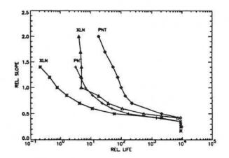
Figure 3 Comparison of life reductions from the extended line contact analysis with full point contact calculations for two dents,  $f_X = 0.50$  and  $f_X = 1.0$ , as a function of the relative slope  $f_Z/f_X$ .  $p_h = 3.0$ GPa, b = 0.3 mm, a/b = 8, smooth contact life is  $0.8513 \ 10^4$ .
