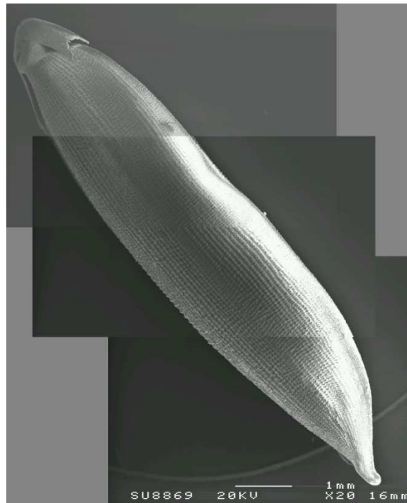
Figure 7 Electron Micrograph of Long Grain Rice Husk (composite image)
