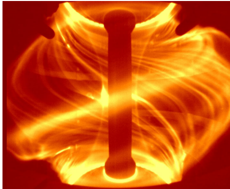
Figure 4.2: A Mega Ampère Spherical Tokamak shot showing plasma filaments or blobs during an edge localised mode (Kirk, 2012).
