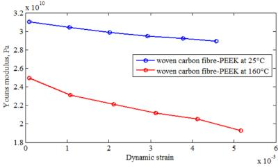
Figure 6: Strain sweep modulus results for woven composite material.
