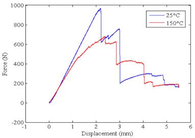
Figure 3: Force-displacement behaviour for woven composite material.
