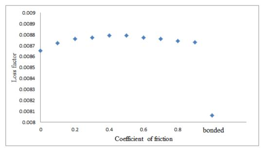
Figure 16: Loss factor at different coefficient of friction.
