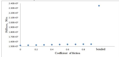
Figure 15: Stiffness at different coefficient of frictions.
