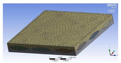
Figure 14: Meshing woven composite unit cell.
