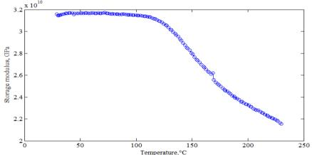
Figure 4: Effects of temperature on flexural modulus for woven composite material.
