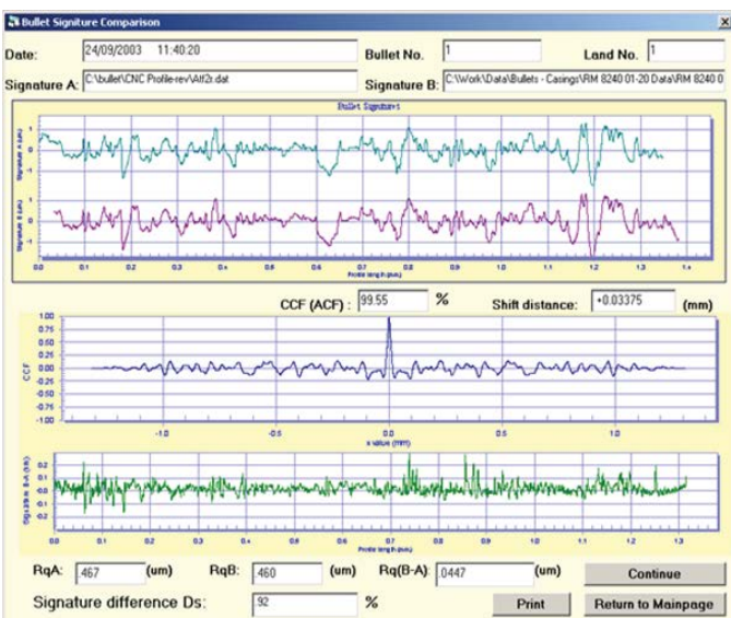
Figure 3 A user screen for bullet signature measurement between the land 1 of SRM 2460-001 Standard Bullet (Signature B, as shown on the second profile from the top) and the virtual standard (Signature A, as shown on the top). The cross-correlation function CCF_{max} = 99.55%, the signature difference D_s = 0.92%. The unite of the top and bottom vertical scales is \mu\text{m} . The unite of the lateral scales is mm.
