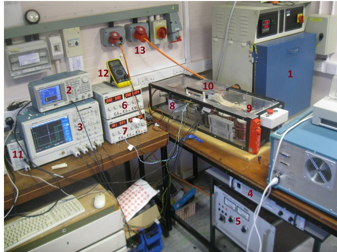
Figure 4: The Inductive clamped Measurement Test Rig including: 1- Environmental Chamber, 2- Signal Generator, 3- Oscilloscope, 4- Main power supply, 5- Interlock power supply, 6- 5V gate driver supply, 7- 18V gate driver supply, 8- capacitors, 9- Inductors, 10- Gate Driver, 11- Probe Amplifier, 12- Safety Volt meter.
