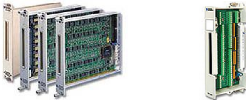
Figure 4.28: (a) SCXI-1102 Voltage input module (b) SCXI-1303 Terminal Block
