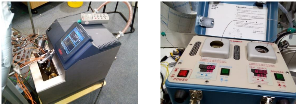
Figure 4.22: (a) Thermocouples in bath (b) Calibration Kit
