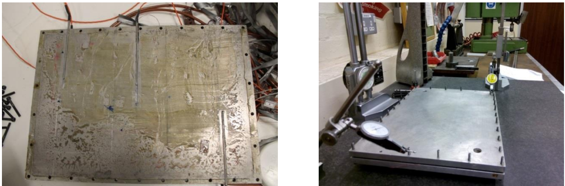
Figure 4.12: (a) Distortion of grease layer (b) Procedure for measuring the sandwich
