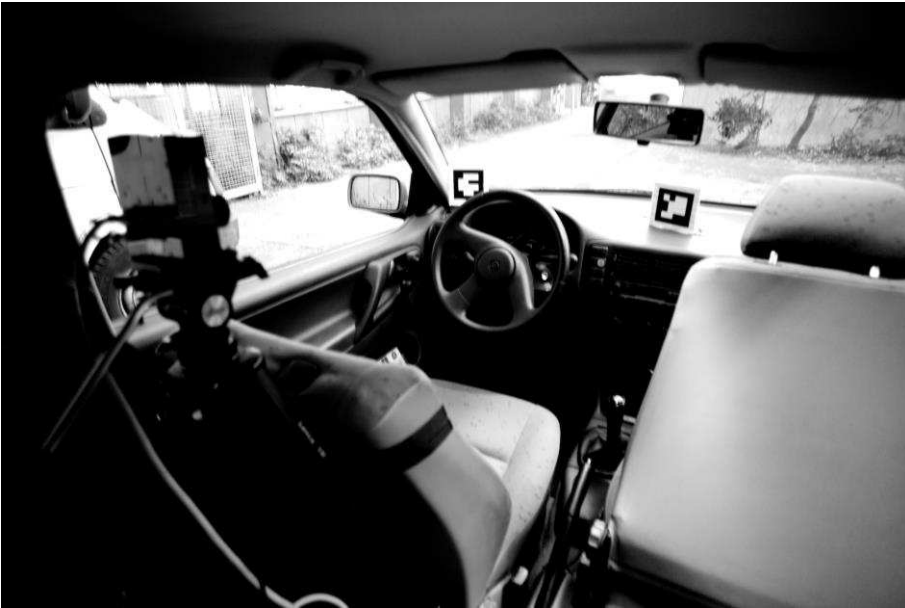
Figure 2. Photograph of the interior of the test vehicle to illustrate the location of the fixed camera (mounted behind the driver's seat) and the augmented reality markers (ARMarkers), here located on the left-hand and right-hand sides of the steering wheel.
