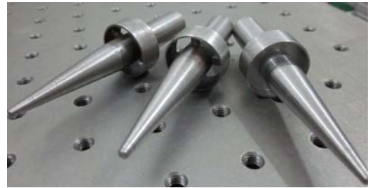
Fig. 13. The concentrators with decoupling flanges.
