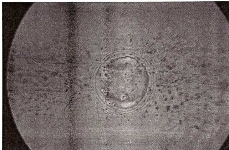
Fig 8 Optical EHD photo of 5 micron silicon carbide particles entering the contact (photograph magnification \times 60 , photographically reduced to 55 percent)
