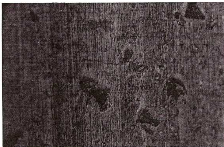
Fig 10(b) Photomicrograph of raceways tested with SiC contaminated lubricants (photograph magnification \times 300 , photographically reduced to 55 percent)
