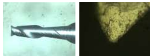
Fig.10 Microscopic picture of WC micro-mill cutting tool
