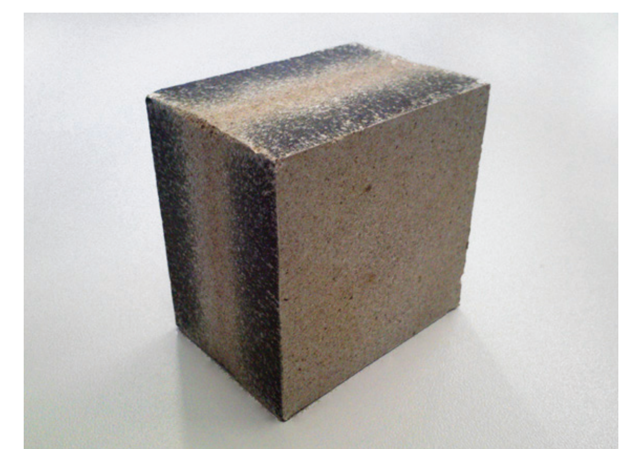
Fig. 3 – Dry sand specimen after compression to 800 MPa.
