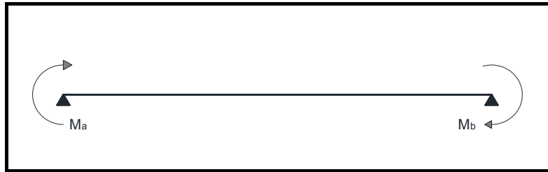
Figure 6.1 – Beam subject to a variable linear bending moment.
