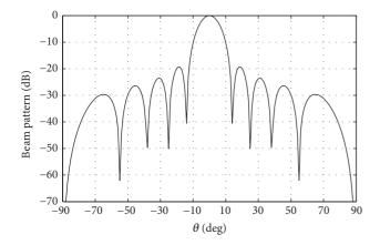
FIGURE 2: Beam response for the design example based on a ULA.
