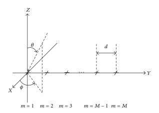
FIGURE 1: Array model being considered with crossed dipole elements.
