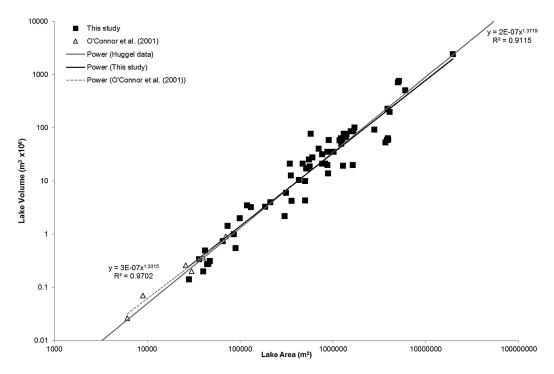
**Figure 2.** Plot of lake area against volume for the data compiled in this study and for the data presented by O'Connor et al. (2001). Best-fit lines and corresponding equations and  $r^2$  values are presented for both data sets. The solid grey line represents the area—volume relationship of Huggel et al. (2002) (Eq. 3) for reference.
