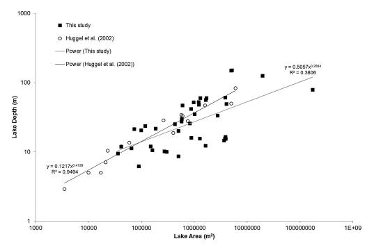
**Figure 1.** Plot of lake area vs. depth for the data compiled in this study (including duplicate measurements of individual lakes) and the data presented by Huggel et al. (2002). Best-fit lines and corresponding equations and  $r^2$  values are presented for both data sets.
