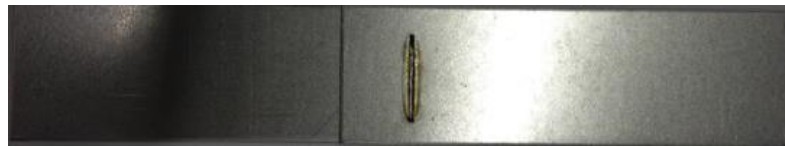
Figure 4.6: Transverse linear weld by RLW on overlapping coupons
