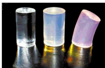
Fig. 10 Left: pure polystyrene polymer cylinder; middle: hard polymer material containing both polystyrene and a LMWG network; right: rubbery polymer containing poly(2-ethyl hexyl methacrylate). Image reproduced from reference 30b with permission from Wiley-VCH.
