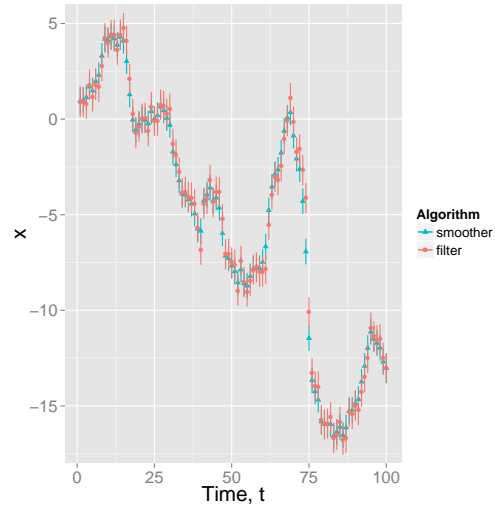
(b) Exact filter and smoother: points show the mean, vertical bars the extent of \pm 1 standard deviation intervals.
