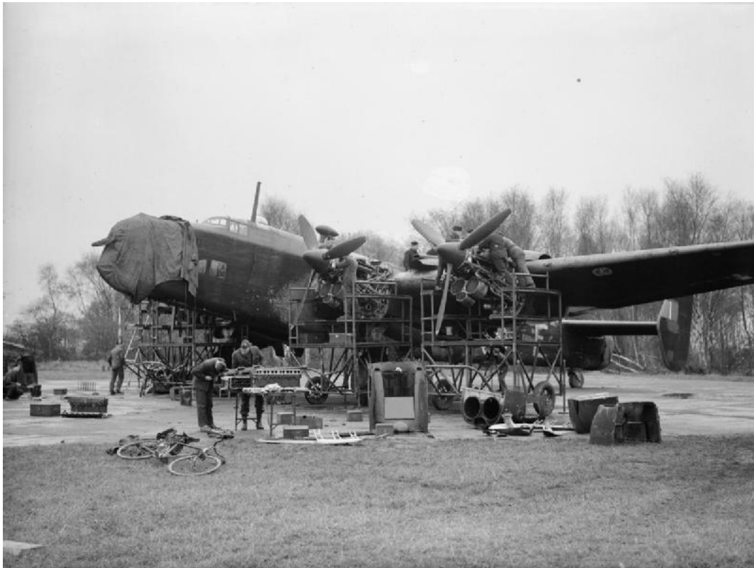
FIG 3.3. Ground crews overhaul the Rolls-Royce Merlin XX engines of Handley Page Halifax Mark II, BB194 'ZA-E', of No. 10 Squadron RAF, in a dispersal at Melbourne, Yorkshire, IWM, CH 7910.
