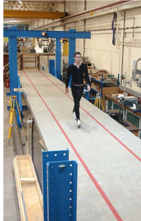
Figure 14. A walking test on the Warwick Bridge.
