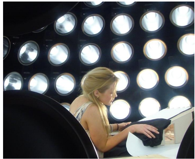
Figure 3: Point Source Artificial Sky Dome. Photo taken at University College Dublin, November 2011
