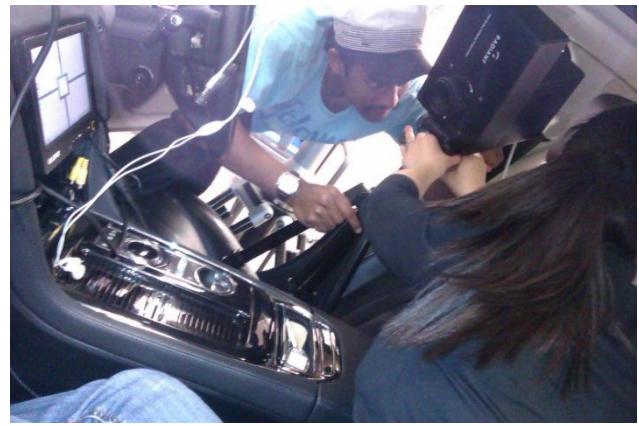
Figure 5: Typical set-up for in-vehicle display assessments based on ISO 15008 [6] and SAE J1757-1 [7]
