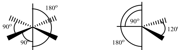
Figure 3.1; Left the octahedral geometry with two unique A-M-A angles and right a trigonal bipyramidal geometry with three unique angles. 97
