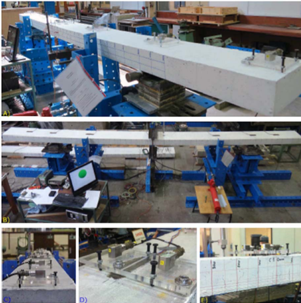
Figure 4: Experimental setup: (a) RC Beam 4 with accelerometers; (b) RC Beam 5 with the load cell installed at the mid-span; (c), (d) and (e) installed accelerometers and typical pattern of flexural cracks near the mid-span point.
