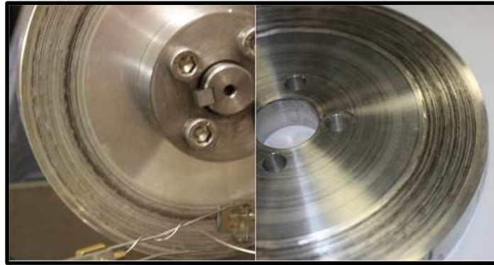
Figure 4: Uncoated aluminium alloy rotor after test showing badly degraded rubbing surface
