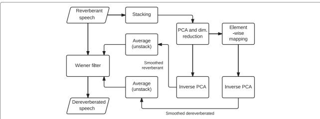
Fig. 2 Distribution matching (DM) flowchart. An overview of the DM dereverberation process. Here, the reverberant speech input and dereverberated speech output are represented as Mel-spectral feature vectors
