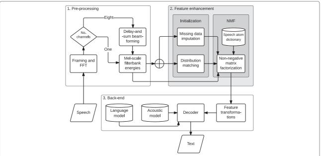
Fig. 1 General flowchart of the feature enhancement method and back-end ASR system. Overview of the speech signal processing pathway from time domain audio to decoding and recognition hypothesis
