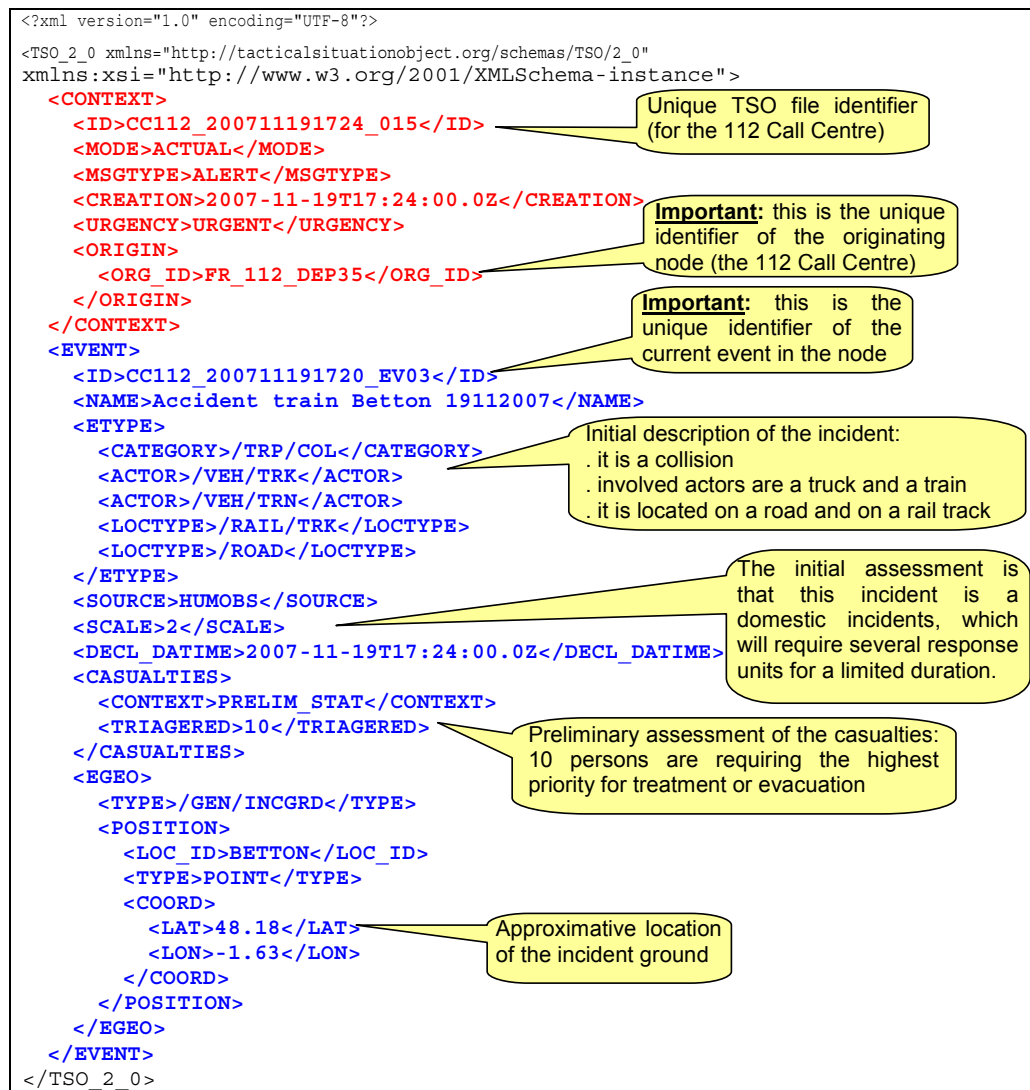
Figure 6.1: A Tactical Situation Object (TSO) Created by the Emergency Services Call Centre [43]
