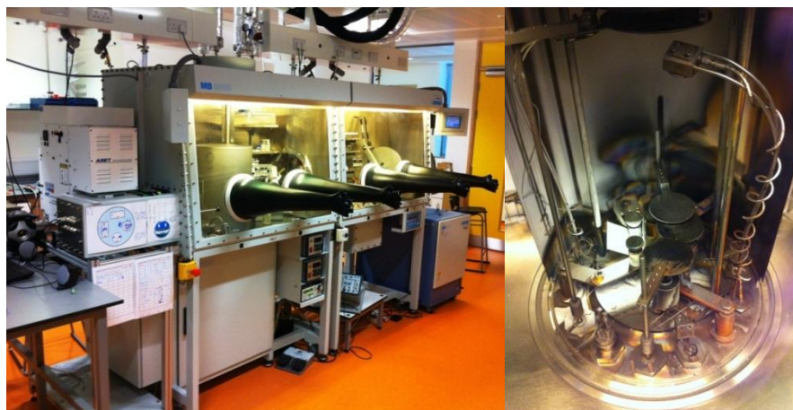
Figure 2.12: The MBraun MB 20G LMF Glovebox (left) with solar simulator (far left) and the CreaPhys Organic molecular evaporator (right) used.
