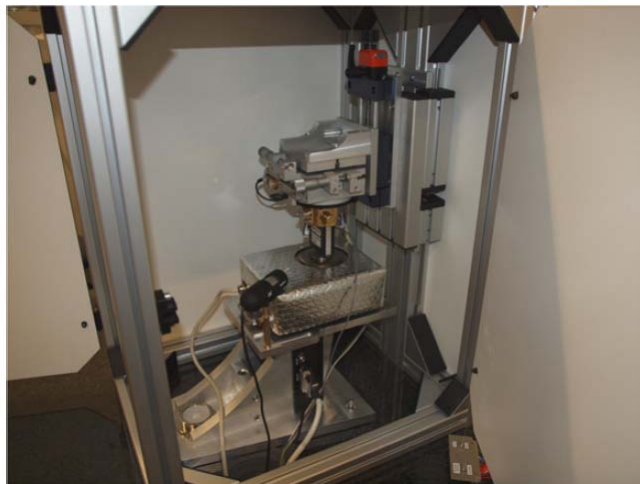
Figure 2.12: Photograph of the new FSM. In the lower part one can see the NPT and the balance, surrounded by a foil to reduce thermal influences. Above the balance, the transducer, with the adapter mounted on the rotational and tilt table (from [8]).
