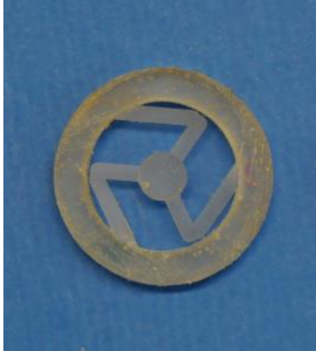
Figure 5.9: The sample ABS1-60 of a angle-beam triskelion force artefact with elbow angle 60^\circ .
