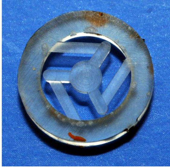
Figure 5.3: The sample CS1-60 of a classic triskelion force artefact with elbow angle 60^\circ .
