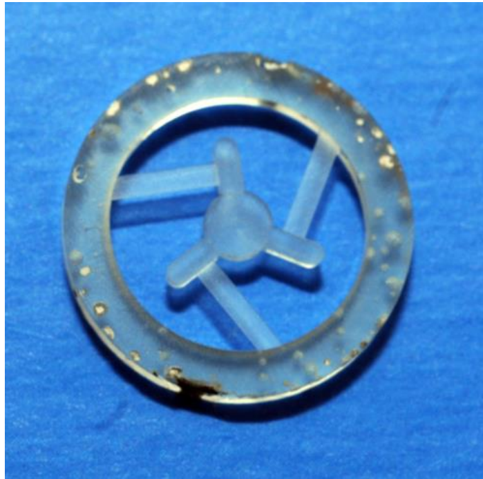
Figure 5.5: The sample CS1-90 of a classic triskelion force artefact with elbow angle 90^\circ .
