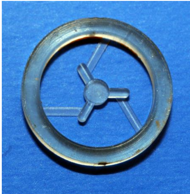
Figure 5.7: The sample CS2-120 of a classic triskelion force artefact with elbow angle 120^\circ .
