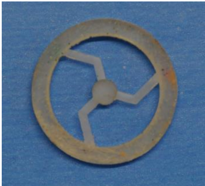
Figure 5.8: The sample ABS2-120 of a angle-beam triskelion force artefact with elbow angle 120^\circ .
