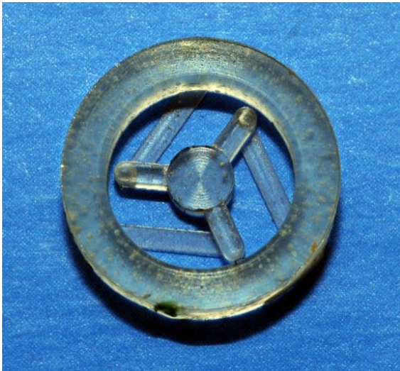
Figure 5.4: The sample CS2-604 of a classic triskelion force artefact with elbow angle 60^\circ .
