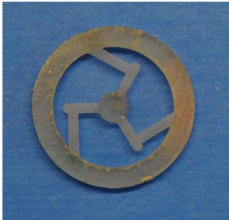
Figure 5.6: The sample ABS2-90 of a angle-beam triskelion force artefact with elbow angle 90^\circ .
