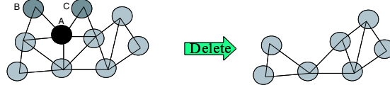
Figure 2.5: Figure illustrating cell deletion. Cell A is deleted. Cells B and C are within the neighbourhood of A and would be left dangling by the removal of the five connections surrounding A so B and C are also deleted.
