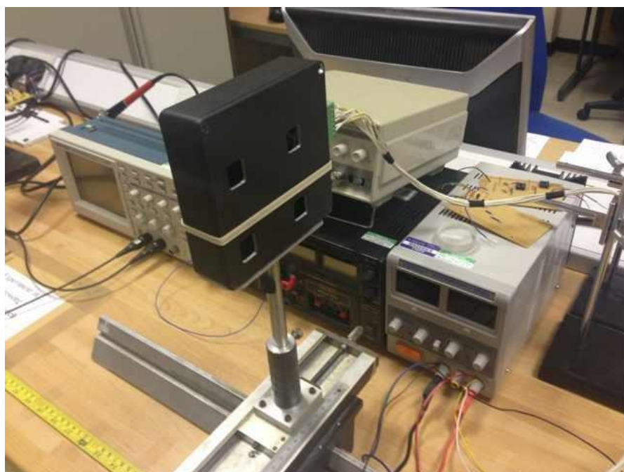
Figure 4-18 Receivers of Infrared OOK MIMO system
