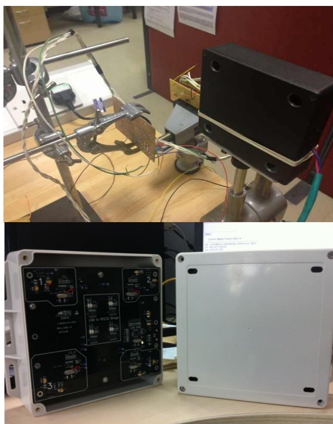
Figure 4-19 (Up) OOK MIMO Transmitters; (Bottom) 4PPM MIMO Tranceivers
