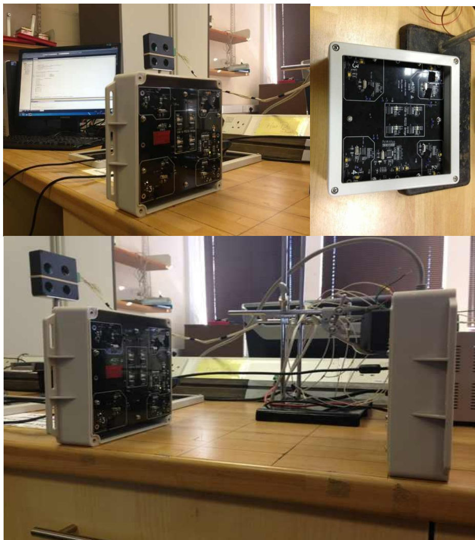
Figure 5-3 4PPM and SIR Transmitters and Receivers (4X4 Transceivers)
