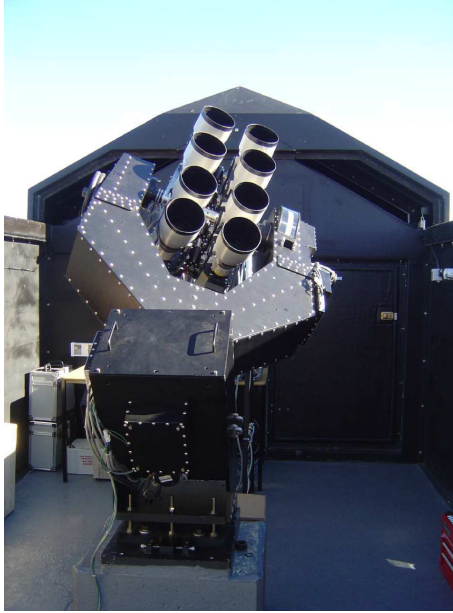
Figure 1.6: One of the two SuperWASP instruments [Pollacco et al., 2006], here shown at the South African Astronomical Observatory.
