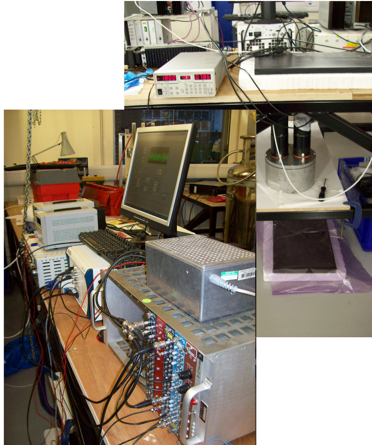
Figure 3.19: The optical readout detector system: Left, the PMT power supply, data acquisition system, and NIM crate, and Right, PMT power supply, the detector, and two muon paddles.
