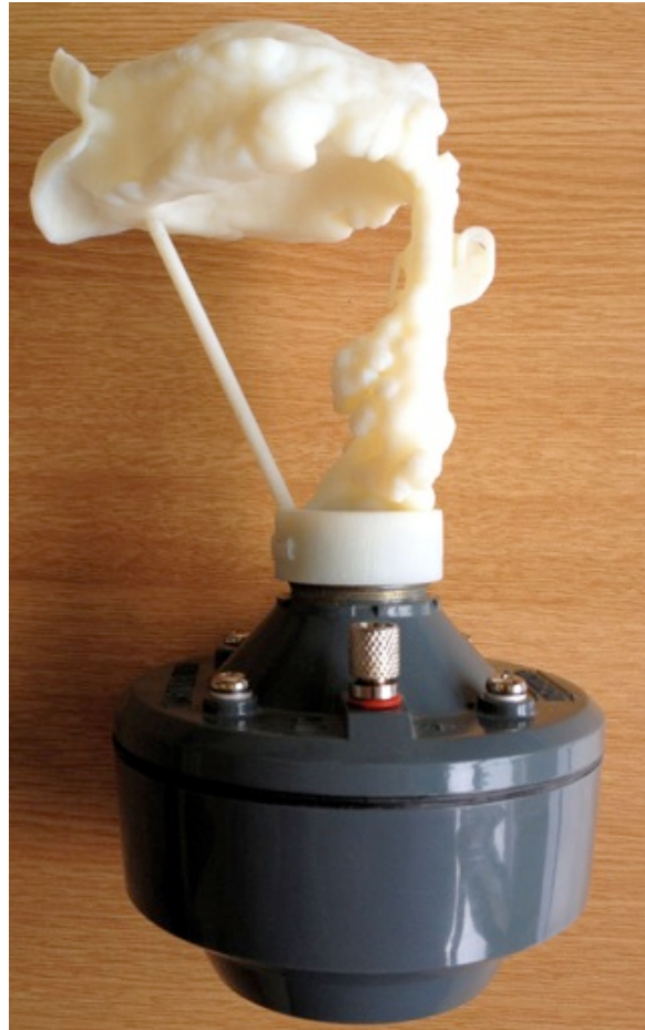
Figure 3: A 3-D print for the vowel “ah” sitting atop its loudspeaker drive unit as used in the Vocal Tract Organ.
