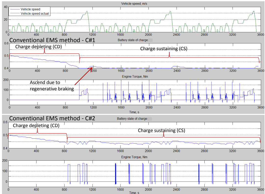
Figure 9-1: Engine performance and SOC profile of conventional EMS methods, C#1 and C#2 over the NEDC 3x with initial SOC of 0.5
