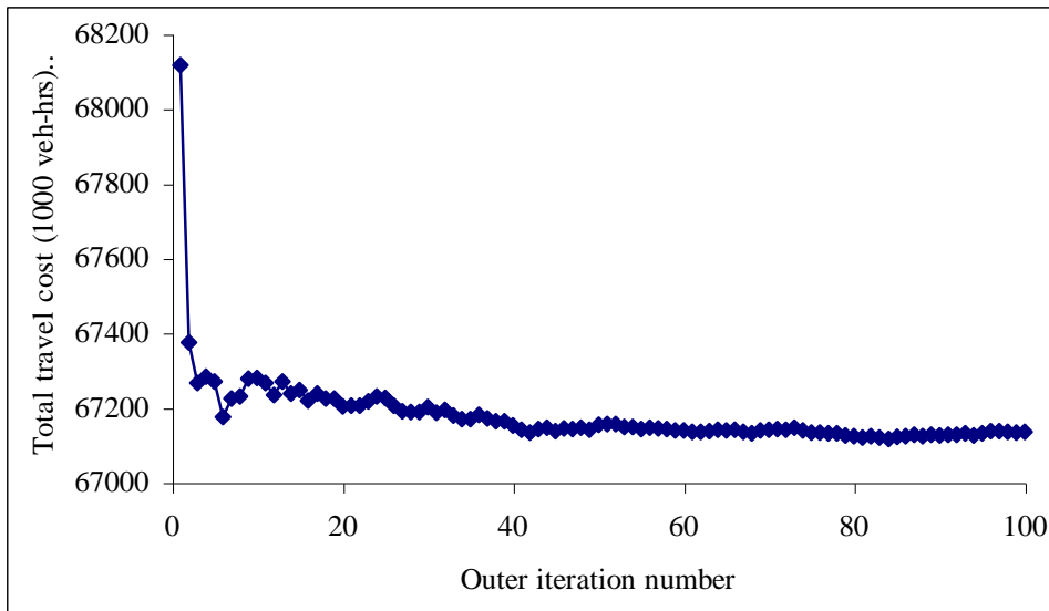
Figure 2: Total travel cost versus outer GSUE(2) iteration (Weetwood network: \tau = 0.1 ; \omega = 0.3 ; 100 inner iterations per outer iteration)
