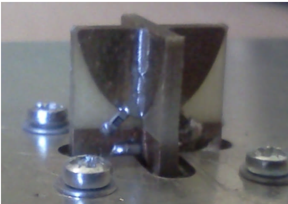
Figure 17. Close up of quad blade antenna
