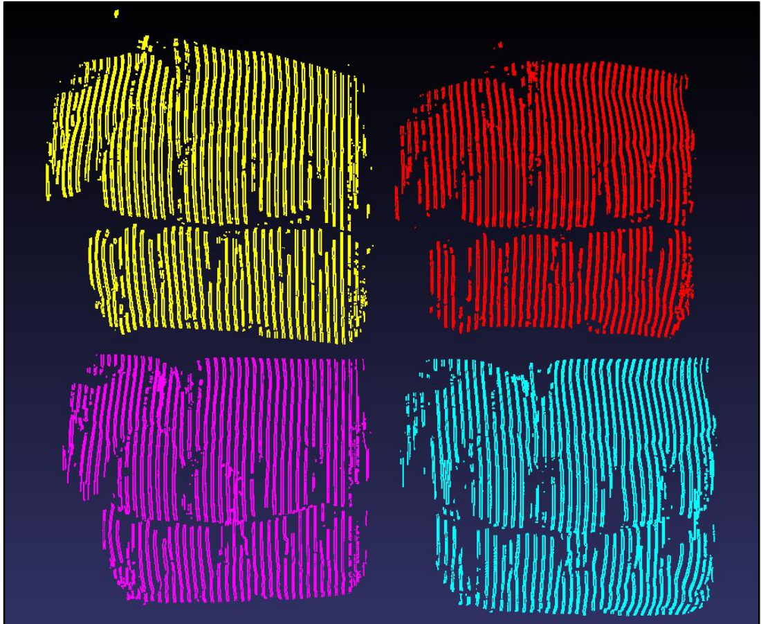
Figure 114 Four Scans from the LM Set. The 1 st (yellow), 11 th (red), 20 th (magenta) and 30 th (cyan) scans from the lateral excursion model set are shown. The quality of the data decreases over the course of the scan. (First scan : 66462 points, 30 th scan : 61258 points).
