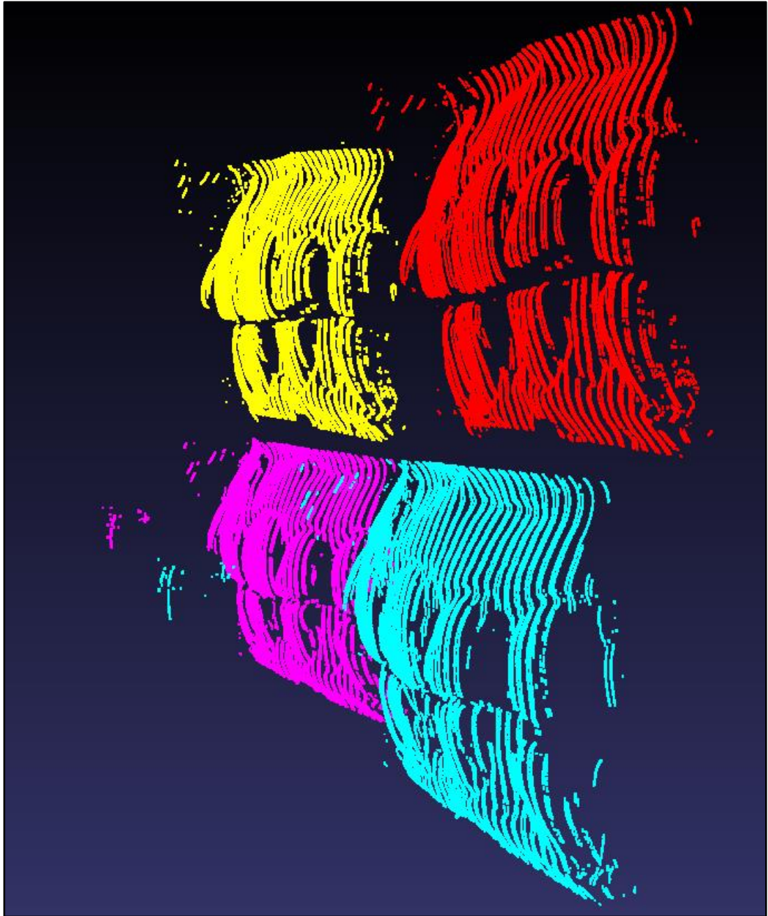
Figure 115 The Jailbar Scan Data for LM, Viewed from the Side. The same data as shown in Figure 114. It can be seen that, in addition to losing data over the sequence, the noise in the data increases (particularly visible as noisy points in front of the models). Noise errors are propagated through the remaining scans.
