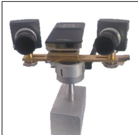
Figure 41 The Cameras and Projector Mounted on a Rigid Brass Bar.
