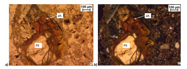
Figure 6.12: Pyroxene (PX) grain altered to an iron-rich alteromorph (alt.) in basalt from sediments adjacent to SK 8 (S1, TS 957), a) PPL and b) XPL.
