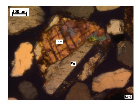
Figure 8.11: Granitic rock fragment, displaying simply twinned feldspar (Pg) and inosilicate (Inos.) components (S1, TS 1240, XPL).
