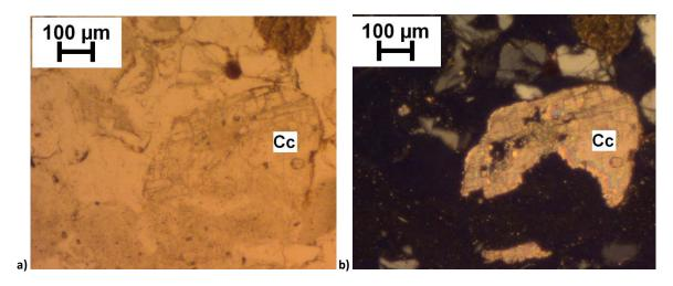
Figure 8.25: Calcite (Cc) which has lost a considerable portion of its total volume through *in situ* weathering processes, a) PPL and b) XPL (C3A, TS 1207).
