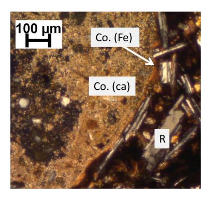
Figure 6.17: Basaltic clast (R) from a control sediment showing a thin iron-rich hypocoating (Co. (Fe)) followed by a thick carbonate-rich coating (Co. (ca)) (C3, TS 1113, XPL).
