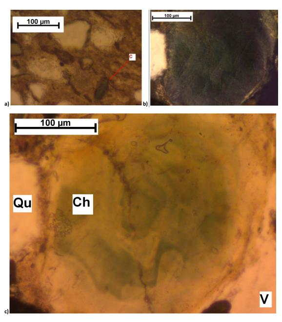
Figure 7.15: Chlorite in thin section from samples. (a) Secondary chlorite (C) with diffuse edges (GR 7555, S2, TS 821.2, PPL). (b) Chlorite (Ch) adjacent to quartz (Qu) and voids (V) (GR 5914, S1, TS 995) (XPL). (c) PPL view of image b) (GR 5914, S1, TS 995, PPL).
