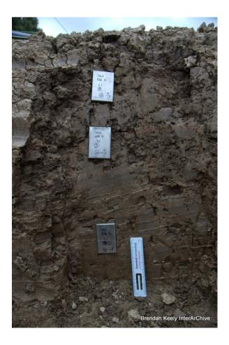
Figure 7.1: The C1 control profile with Kubiena tins in place for micromorphology sampling (C1A, C1B, and C1C).
