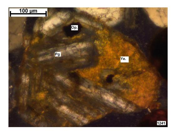
Figure 8.10: Granitic rock fragment, displaying plagioclase feldspars (Pg), opaque material (Op.), and a yellow alteration product (Ye.) composition (S1, TS 1241, XPL).
