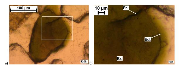
Figure 8.29: Slightly developed weathering of glauconite from controls above the coffin. a) Glauconite with pellicular weathering (C3C, TS 1208, PPL). b) Detail from inset (white rectangle) in image a) showing intra-mineral fracture (Fr.) extending from the upper edge of the grain into the mineral, diffuse edges (Ed.) and a brown colour (Br.) in the lower portion of the field of view (C3C, TS 1208, PPL).
