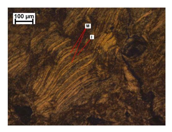
Figure 7.12: Holo-meso-alteromorph of biotite (M) showing expansion between sheet-like layers (I), following a parallel linear weathering pattern leading to the production of clays (GR 7519, C3, TS 875, XPL).
