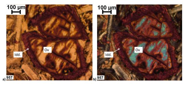
Figure 6.11: Olivine (Ov) within basalt from the sediments adjacent to SK 8 (S1, TS 957), a) PPL and b) XPL. The associated iddingsite (Idd.) is interpreted as due to alteration, and not as a result of weathering occurring in the sediments.
