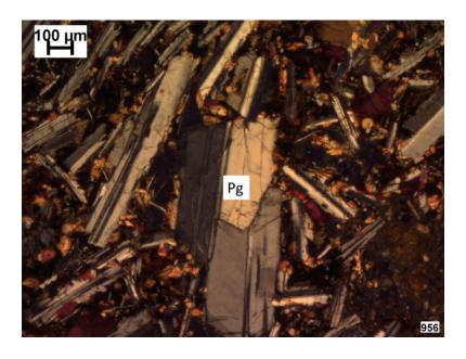
Figure 6.10: Plagioclase (Pg) phenocrysts in basalt from the sediments surrounding SK 5, containing plagioclases of both simple and polysynthetic twinning (SK 5, S1, TS 956, XPL).
