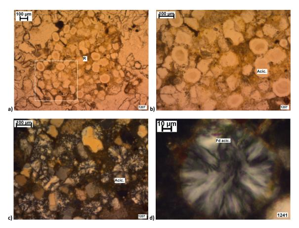
Figure 8.27: Fibrous chalcedony. a) Rock (R) composed of fibrous chalcedony and yellow fine material (C3A, TS 1207, PPL). b) Detail of inset from image a), showing fibrous chalcedony (Acic.) and yellow fine material (C3A, TS 1207, PPL). c) XPL view of image b) (C3A, TS 1207, XPL). d) Fibrous chalcedony observed in a skeletal adjacent sample which is not held within a rock fragment (S3, TS 1241, XPL).
