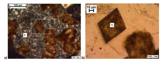
Figure 8.12: a) Rock fragment (R), composed largely of minerals displaying first order grey interference colours and with titanite as an accessory mineral (C4A, TS 1163, XPL). b) Detail of titanite (Tt) from within inset (white rectangle) in image a) displaying brown colour (PPL) and very high relief of titanite (C4A, TS 1163, PPL).
