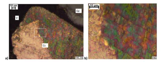
Figure 8.13: a) Calcite (Cc) displaying pellicular weathering at edges (left side of field of view) and rhombohedral structure as shown through the visibility of all three cleavage planes, adjacent to quartz (Qz) and voids (V) (C4A, TS 1163, XPL). b) Detail of inset from image a) (C4A, TS 1163, XPL).
