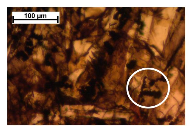
Figure 6.14: Opaque secondary products, displaying diagonal cubic morphology (circled in white) (SK 8, S1, TS 1112, PPL).
