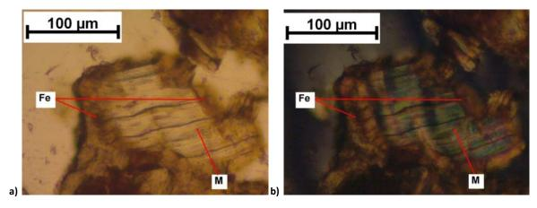
Figure 7.18: a) Mica (M) with mineral weathering at tops and bottoms of the mineral grain, through pellicular weathering with deposits of iron oxide compounds precipitated out of solution (Fe) (GR 5914, SA2, TS 906, PPL). b) XPL view of image a).
