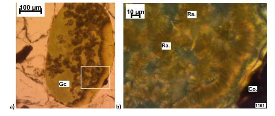
Figure 8.34: Slightly weathered glauconite from sediments within the coffin. a) Glauconite (Gc) was well preserved (C4B, TS 1161, PPL). b) Radially structured (Ra) surficial impressions formed during the primary (marine sourced) formation of the mineral remain visible, with slight weathering effects observed via the opaque coating (Co.) which has been deposited post-rounding of the grain (C4B, TS 1161, XPL).
