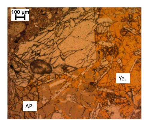
Figure 6.13: Glassy groundmass displaying grey colours and altering to a yellow coloured product in basalt from the sediments surrounding SK 1 (SK 1, S1, TS 965, PPL).
