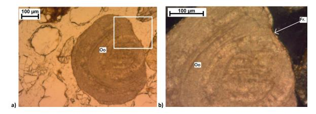
Figure 8.24: Ooid in thin section from control C3A (TS 1207). a) Ooid (Oo) displaying concentric rings and grey colour (C3A, TS 1207, PPL). b) detail from inset in image a), showing the fractured edges (Fr.) of the ooid (Oo) which were first fractured, then rounded, and subsequently weathered through pellicular weathering (C3A, TS 1207, XPL).
