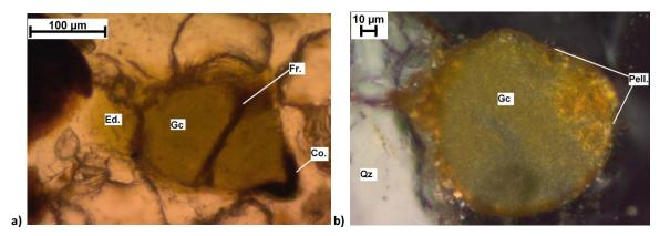
Figure 8.31: Moderately developed weathering of glauconite from C3 controls. a) Glauconite (Gc) with dark coloured partial coating (Co.), transmineral fracture (Fr.) and diffuse edges (Ed.) (TS 1208, C3C, PPL). b) Glauconite (Gc) of well-rounded form and small size ( $^{\sim}100~\mu m$ ) with pellicular weathering (Pell.), and surrounded by quartz (Qz) (C3C, TS 1208, XPL).
