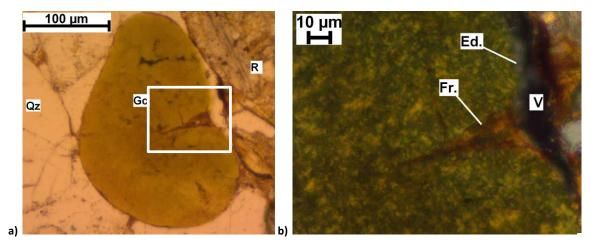
Figure 8.30: Moderately developed weathering of glauconite from controls. a) Glauconite (Gc) has altered to a brownish-yellow colour, adjacent to quartz (Qz) and rock fragments (R) (C4B, TS 1161, PPL). b) Detail of inset (white rectangle) in image a), showing diffuse edges (Ed.) near a small void (V) and an intra-mineral funnel-shaped fracture (Fr.) extending from the edge of the grain (C4B, TS 1161, XPL).
