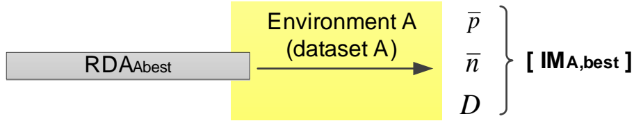
Figure 5.6: Calculation of the reference implicit vector. The implicit vector is associated with a specific RDA and a specific environment on which it is calculated. When an RDA runs through a specific dataset/environment, a log of the position and negative feedback values along with details about the output detections can be used to calculate an implicit performance vector for the RDA. The reference implicit vector, IM_{A,best} is the one that corresponds to the best trained RDA, RDA_{A_{best}} on the training data (environment A under the current notation).
