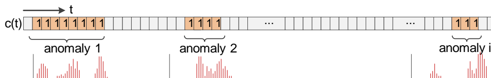
Figure 2.7: A minimal representation of the output of RDA. At every timestep (with every new reading), the RDA outputs a classification signal. The start of an anomaly is the first timepoint where the position of any receptor exceeds 1, resulting in a classification signal of 1. The end of an anomaly is the first timepoint where every receptor has fallen below the detection threshold. Therefore, one anomaly takes place over a number of consecutive timepoints (duration). The first - anomaly detection - level of the RDA is the binary, classification signal output, indicating the presence or not of anomalies. For the second level - identification -, a signature is extracted for every anomaly and this signature can be used to recognise the anomaly.
