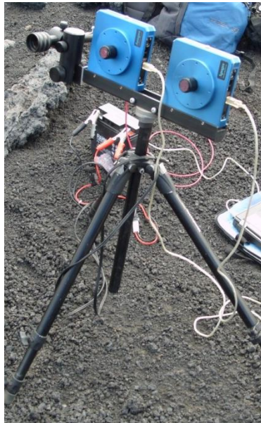
Fig.1.7: The Apogee Alta U260 two camera , two filter, set-up. A cylindrical lens DOAS is also attached to aid with the calibration procedure.
