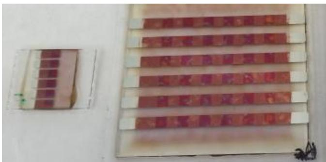
**Figure 4-21: A photograph displaying the small 6 pixel and large 36 pixel architectures after full fabrication.**
