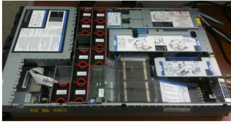
Figure 2.14 An image showing the inside of a typical server, with the internal fans visible and the CPUs located underneath heat sinks (Ibrahim et al., 2012)
