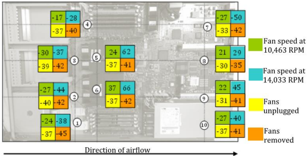
Figure 7.7 Pressure difference (Pa) between a certain point and the server exit for four cases; (a) fan at 10,463 RPM, (b) fan at 14,033 RPM, (c) fans unplugged, and (d) fans removed. Cases (c) and (d) were operated by drawing air through the server using an external fan.
