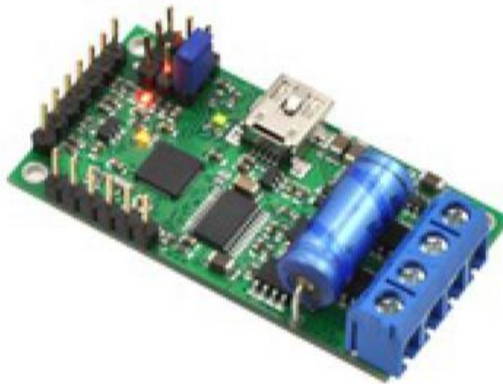
Figure 7.4 Pololu Simple Motor Controller 18v15, with a maximum voltage of 30 V and maximum continuous current of 15 A (Pololu Corporation, 2001)
