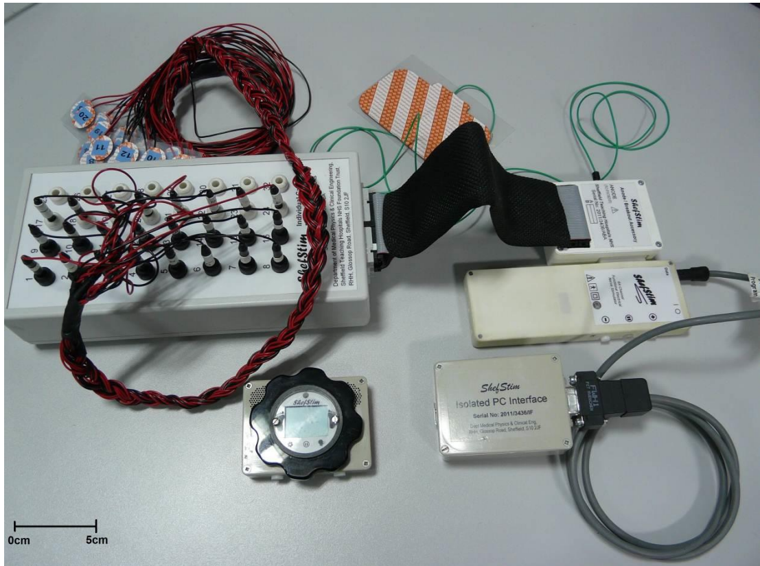
Figure 3.3 The ShefStim system with a breakout accessory box. The overall system consists of the modified stimulator, a remote control, an isolated PC interference and the breakout accessory.
