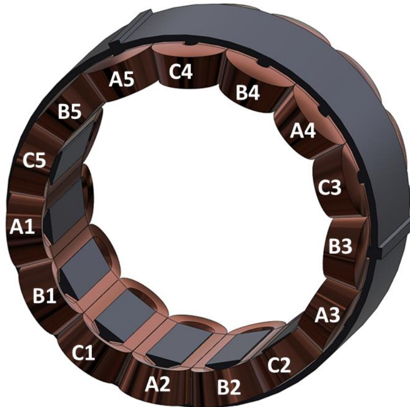
Figure 73 Location of the coils around the stator
