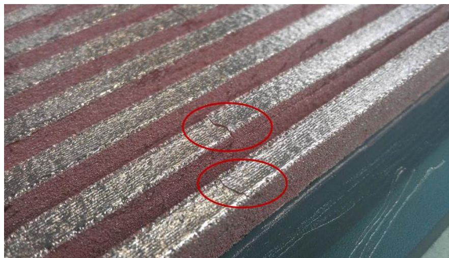
Figure 100 Surface cracks developed in test sample
