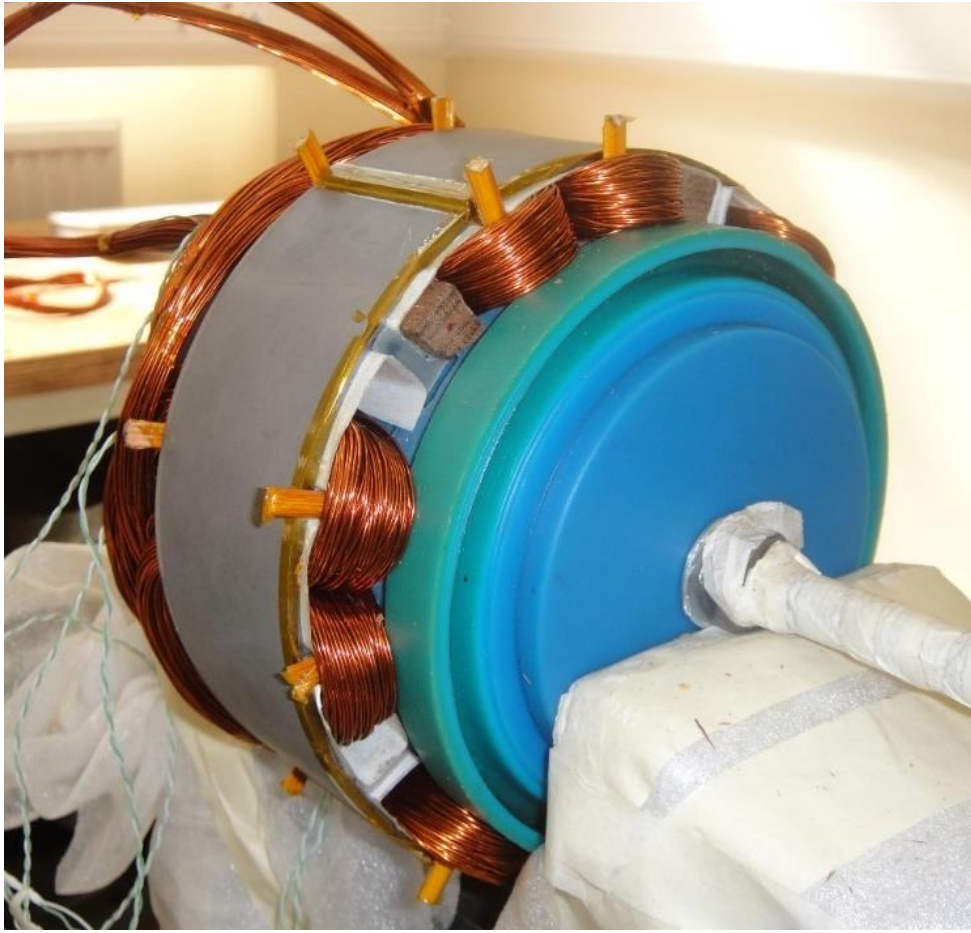
Figure 49 Stator winding part-way through manufacture
