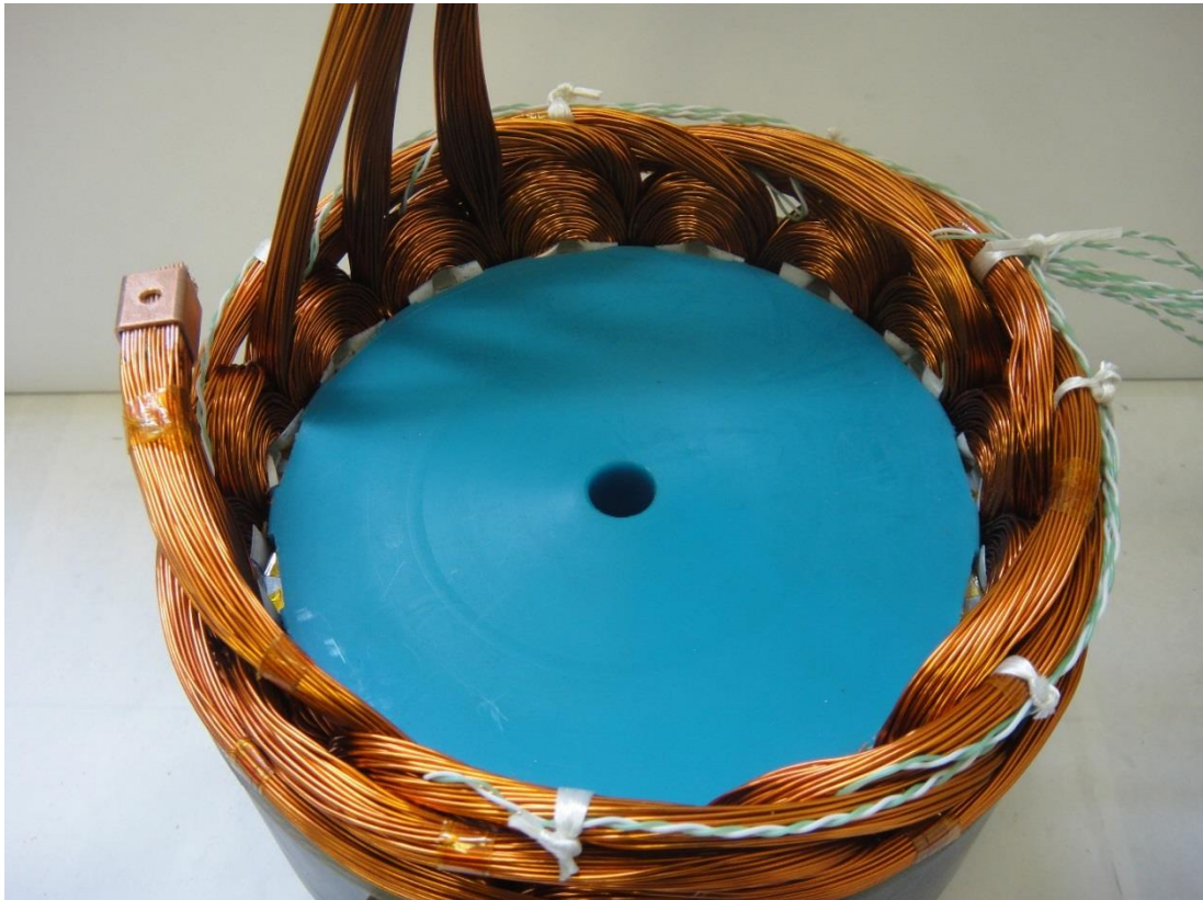
Figure 56 View of interconnections and star-point of completely wound stator
