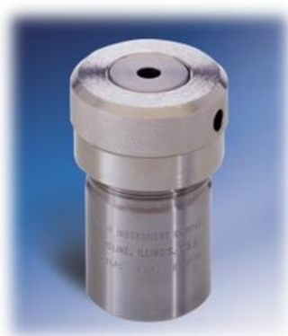
Figure 124 Conventional pretreatment acid digestion vessel (Parr Instruments, Moline, IL)
