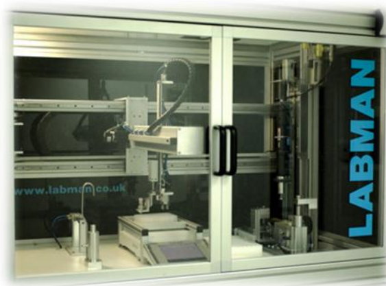
Figure 26 Robotic platform for measuring digestibility of biomass samples
