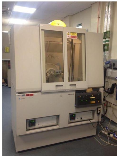
**Figure 3-11** The XRD machines operated in this research: (a) Bruker D8 X-ray diffractometer and (b) Philips Analytical X'pert MPD diffractometer
