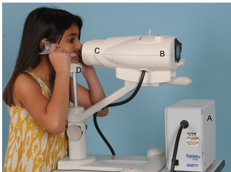
Figure 3.2 Photograph is taken by the IKAM with the patient's chin positioned on the chin rest while the patient is holding the cheek retractors. A is the light box, B is the camera housing, C is the IKAM cone and D is the chin rest.
