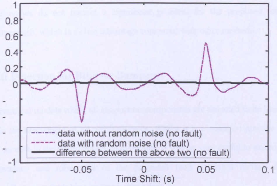
Figure 4.20 CCF coefficient of bounce and pitch accelerations for case 4.9 (no fault)
